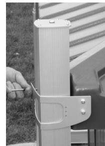
Caution the jack is spring loaded and removal of the pin will allow it to extend, ensure measures have been taken to contain this movement. A tie strap works very well—attach trough the jack ear at the top and to one of the aluminum frame members at the bottom
