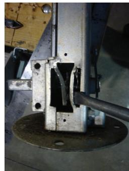
Using a 7/32"/5mm roll pin punch, punch out the roll pin, 6mm x 28mm, that has sheared. There are two sprockets per post and two roll pins, the roll pin in question would be the one furthest away from the square shaft.
