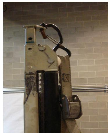
Using a large flat head screwdriver pry and break out the small metal bars to create more space to work
